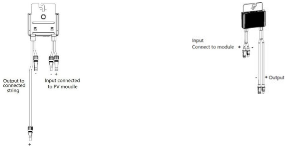
Figure: S-Series (left) and P-Series (right) Power Optimizer connectors
