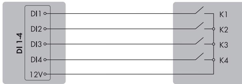
Figure 21: Connect a ripple control receiver to digital input DI 1-4 of the SMA eCharger that is to be configured as System Manager
