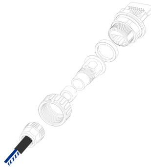
**Figura 2-2** Conector roscado RJ45
