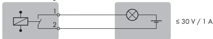
Figure 9: Connection example of consuming device to make contact
