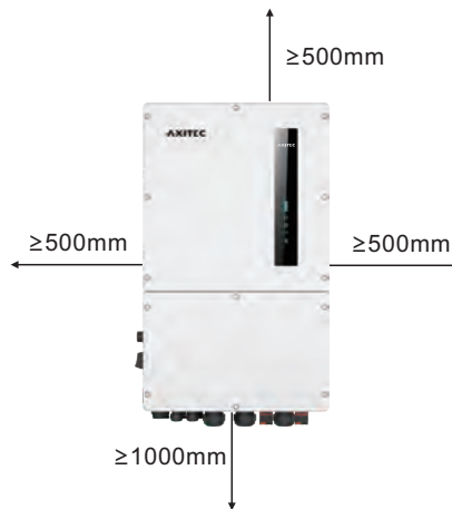
Figure 3.5 Inverter Mounting Clearances
