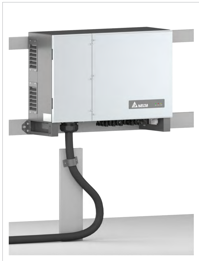
Recommended feeding of the AC cable with strain relief for wall mounting
