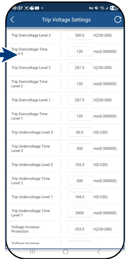
Fig. 116. Define voltage range and shutdown times
