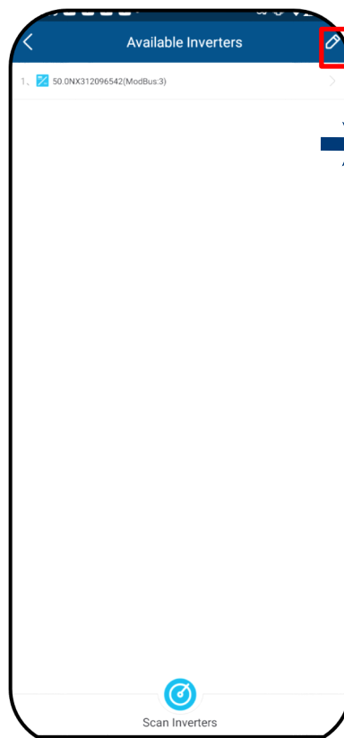
Fig. 88. Opening the Modbus address menu via "Pen"
