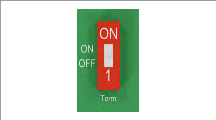
Fig. 7.3: DIP switch for the RS485 termination resistor
