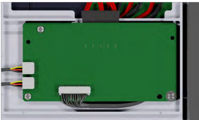
Fig. 4.11: View of the DC surge protection devices with the cover removed
