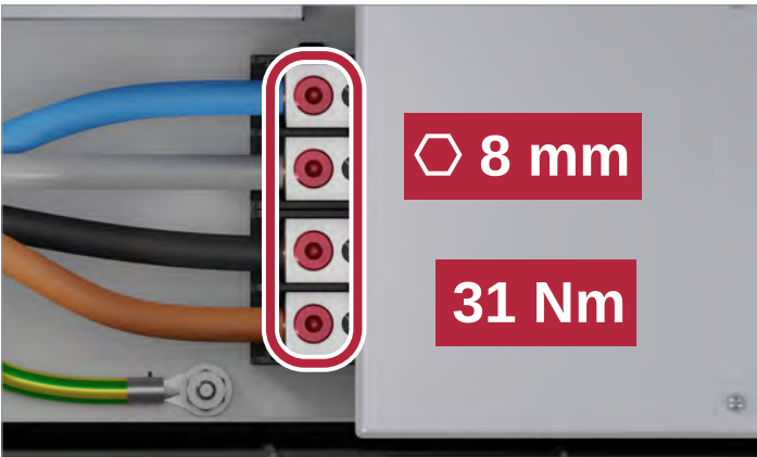
Abb. 6.16: Torques at the AC terminal block
