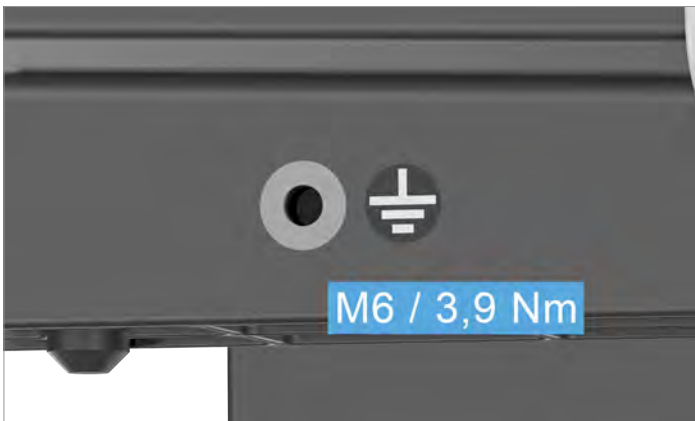
Abb. 6.13: Grounding screw on the left foot of the inverter
