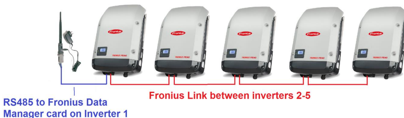
Fig. 7 – Remote Wireless RS485 and Multiple Remote Fronius inverters.
