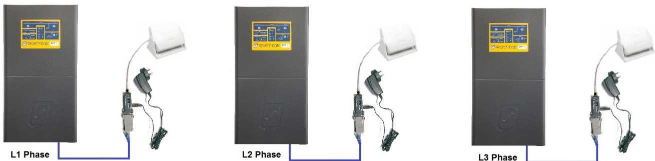
Fig. 6 – Communications wiring for local Wireless RS485 Adaptors in a three phase system.
