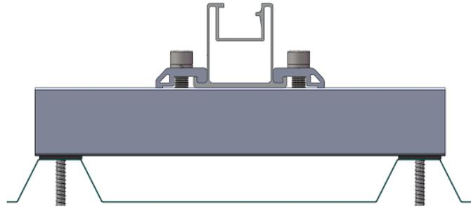
T50/ T110 Rail fix on the top of MT-Rail Support, 240mm
