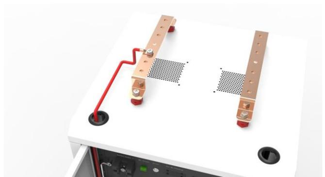
**Step 7:** Connect securely negative terminal of each module with the bottom end of negative output cables. Direct the positive cable up, towards the cabinet's top panel, along the side panel as shown on the picture (below-left), through one of two cable holes in the top panel of the cabinet. Then connect the top end of the negative output cables firmly, by bolt, to the negative busbar installed on stand-off insulators on the cabinet top panel, as its shown on the picture (below-right).
