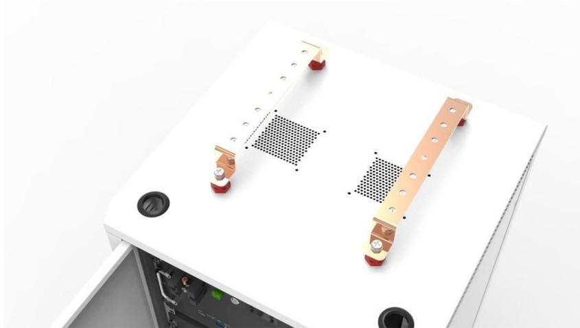
**Step 6:** Connect securely positive terminal of each module with the bottom end of positive output cables . Direct the positive cable up, towards the cabinet's top panel, along the side panel as shown on the picture (below-left), through one of two cable holes in the top panel of the cabinet. Then connect the top end of the positive output cable firmly, by bolt, to the positive busbar installed on stand-off insulators on the cabinet top panel, as its shown on the picture (below-right).
