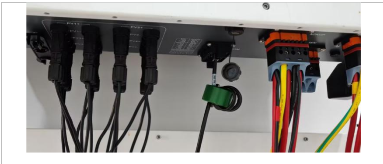
Figure 6-15 Communication cable wound around magnetic ring
