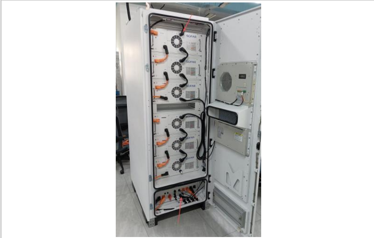
Figure 6-4 Connect the link cable
