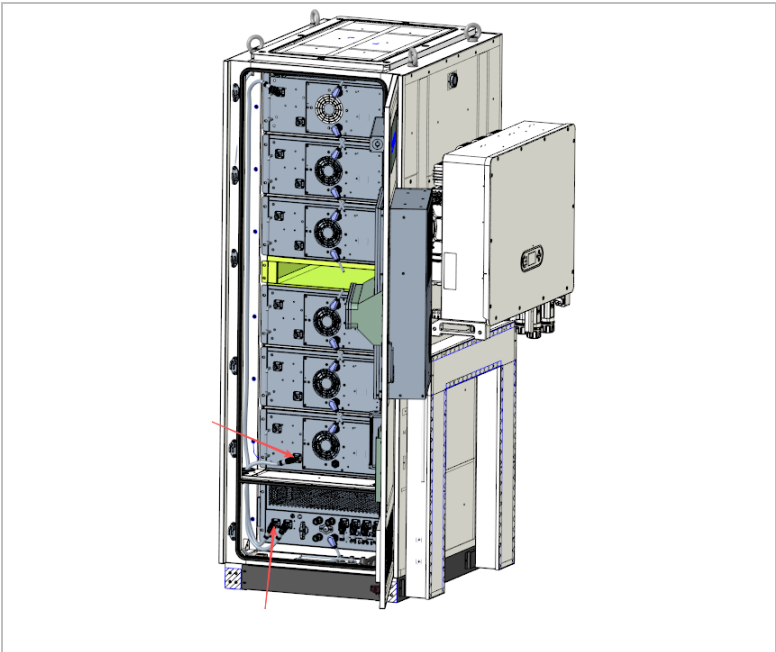
Figure 6-6 Connect the B- power cable between BCU and battery pack
