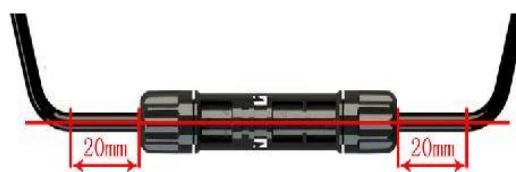
Right way for the cable
