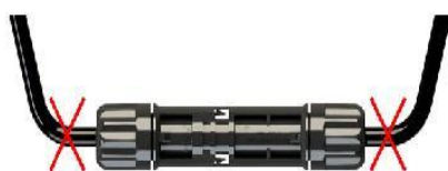
Wrong way for the cable
